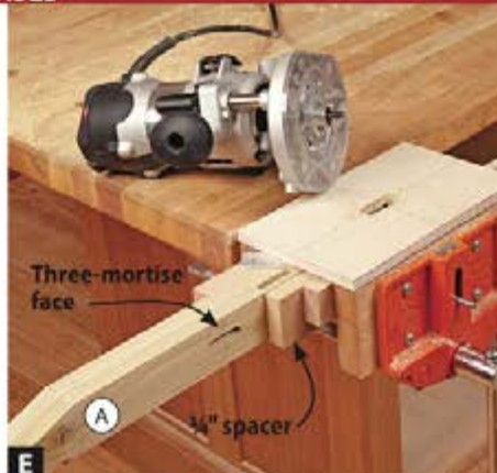
E For the mortises in the adjacent faces, secure the jig to the leg with a \frac{3}{4} "-thick spacer against the three-mortise face.
