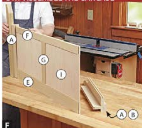
F Working with the parts upside down keeps the top ends of the legs (A) and the edge of the top rail (E) flush during assembly.
