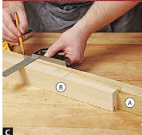
C Clamp together adjacent legs and stiles with their tops flush; then, use a square to mark the centerlines of mating mortises.
