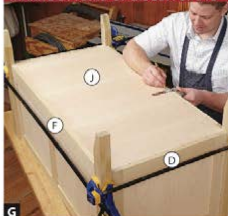
G With a square and pencil, mark across the bottom (J) and adjoining rails about every 6" to locate biscuit cuts.
